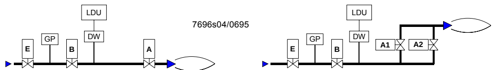
Plants without vent pipe to atmosphere
